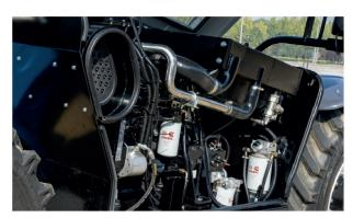
• Independent heat dissipation of Engine and Hydraulic System, through intelligent control logic, timely adjustment of heat dissipation requirements, play a superior role in energy saving. At the same time, the radiatiot fan integrates reverse lowing function, which can effectively remove the debris from the suction outlet.
