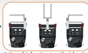
Active safety function: travel lock function If the forks are not in the position, the forklift is actively locked to prevent the operator from accidentally hitting the racks and causing accidents. The above are the three fork safe positions.
